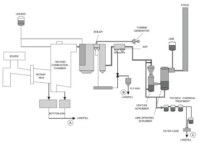
Fig. 1. The plant process diagram and sampling points [14].
